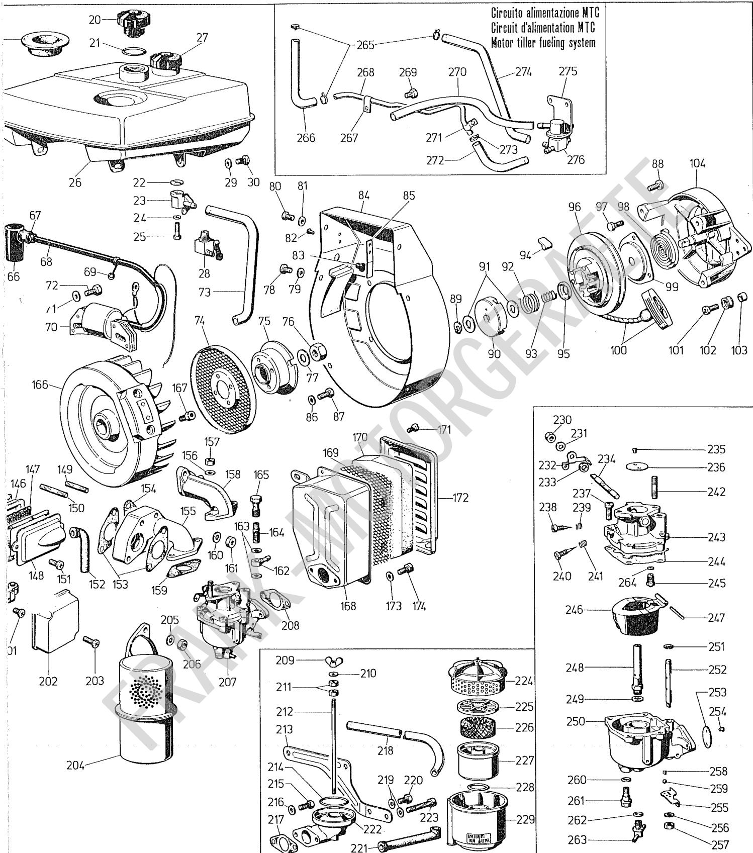
SPARE PARTS FOR ENGINES: STANDARD, WITH REWIND STARTER, WITH OIL BATH AIR CLEANER.
